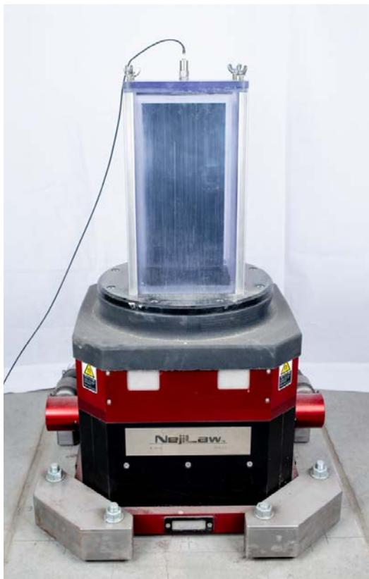
CB elimination device for basic research: Verification of the theory of eliminating CB (Concrete Bubble) generated during concrete placing, discovering new correlations and laws, extract optimal variable inertia force conditions for each blending composition.
