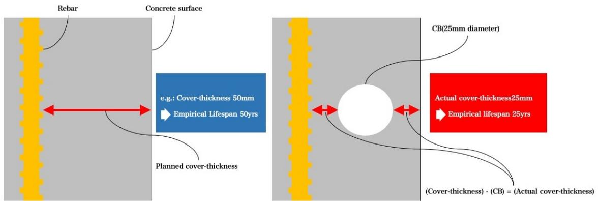
**1** The lifespan of reinforced concrete depends on the concrete cover-thickness. It is assumed that the planned cover-thickness is 50 mm and the empirical lifespan is 50 years.
