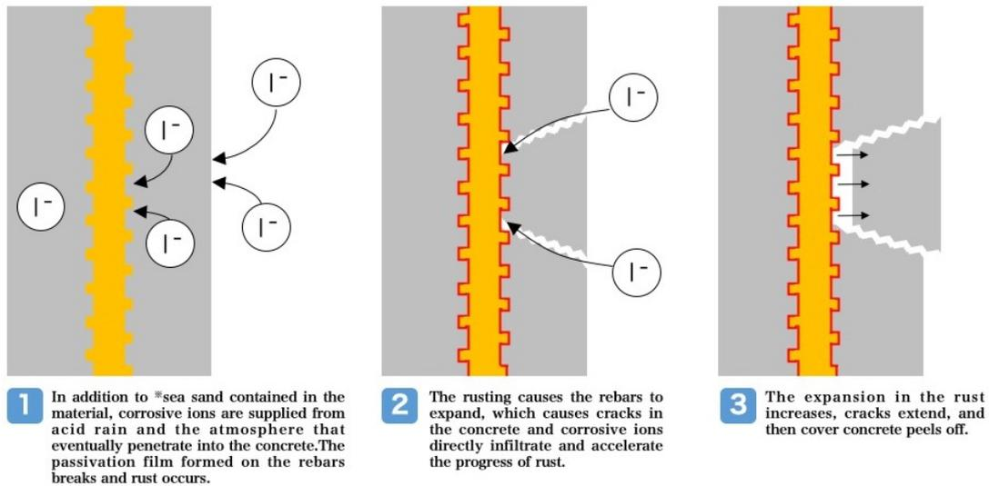
※ In addition to using sea sand as a material, corrosive ions are also supplied from the atmosphere, exhaust gas, acid rain, etc., which penetrate into the concrete and rust occurs due to defects in the passivation film of the rebars.
